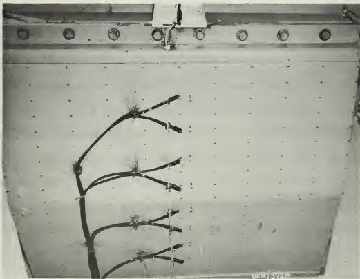
Figure VIII View of Pressure Gages Installed on Model Bottom
